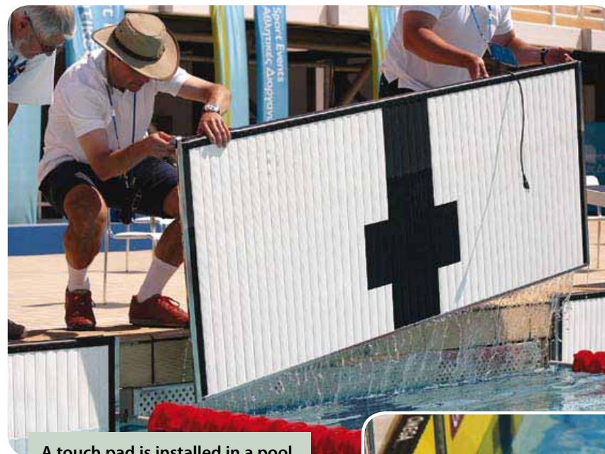
A touch pad is installed in a pool.
